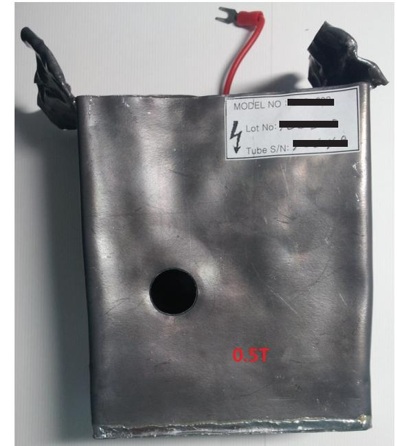
Single layer of poorly wrapped lead - significant leakage radiation detectable from all direction
